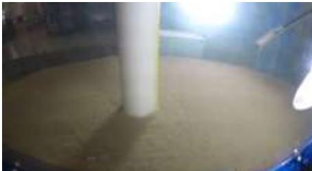
To develop formulas from laboratory experiments for estimation of key parameters, such as the scour depth around piles
